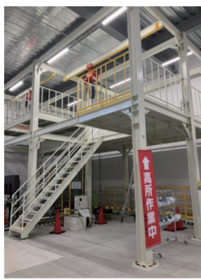
High-place work simulation equipment aligned with Trinity equipment heights
