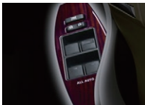
Switch base panel
